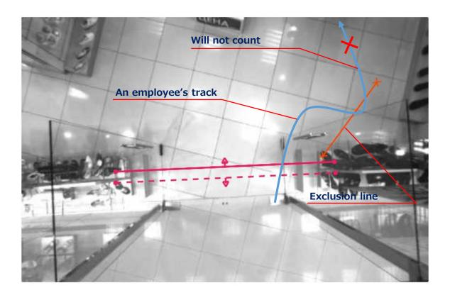
There can be two exclusion lines set up — this way it will be harder for a customer to get excluded from the count. An object will not be counted if crosses both lines in any order (see the diagram below).
